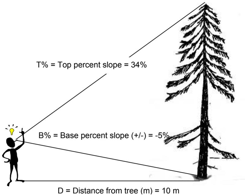
Figure 3. Tree height equals:  $\text{Height (m)} = D \times (T\% - B\%)$ . If the base percent is negative (reading eye-level to tree or on slope above tree DBH), then add B%, if base percent is positive (on slope below tree DBH) then subtract B%.  $\text{Ht} = 20\text{m} \times (0.34 + 0.05) = 7.8 \text{ m}$
