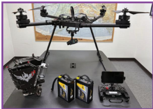
*An Alta X drone with controller (right), two batteries (middle) and the Ignis plastic sphere dispenser that releases plastic balls filled with chemicals used to ignite vegetation on the ground.*
