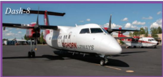
The Alaska Smokejumpers use the CASA 212-200 and the Dash-8. The Dash-8 significantly increases the number of personnel, amount of cargo, response time and range available for initial attack. The CASA carries eight jumpers, referred to as a “load of smokejumpers,” while the Dash-8 can carry 12 smokejumpers. Each
