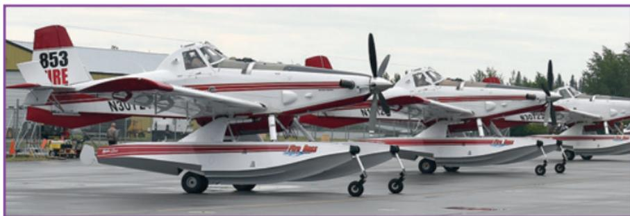
The Air Tractor-802F is a single-turbine, purpose-built aircraft used for water bombing. The AT-802F is powered by one Pratt & Whitney PT-6 with 1,350 or 1,600 horsepower. BLM AFS annually contracts four of these single engine water scoopers at the beginning of the fire season.
