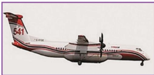
The Conair Q-400AT is a Dash 8-400 converted to a Type 2 air tanker. The Q-400 AT is a high capacity, fast, fuel-efficient and flexible firefighting aircraft designed to replace the CV-
